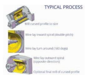
The SWL (saddle wire laying) is an horizontal format, 5-axis CNC controlled electrofusion wire laying machine, designed for machining and wire laying the curved profile of saddle fittings.
