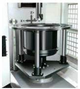
The VWL 400 is a vertical format, 3-axis, CNC controlled electrofusion wire laying machine, designed for the wire laying of medium to large fittings or pipe sections.
